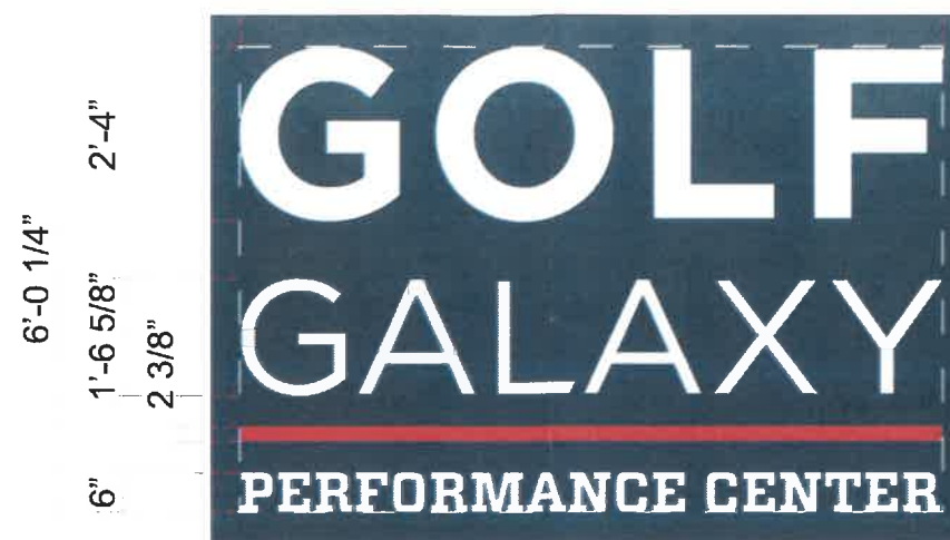
Sign Detail (A.2) - 200 Sq Ft Option Scale: 3/8" = 1'-0"
