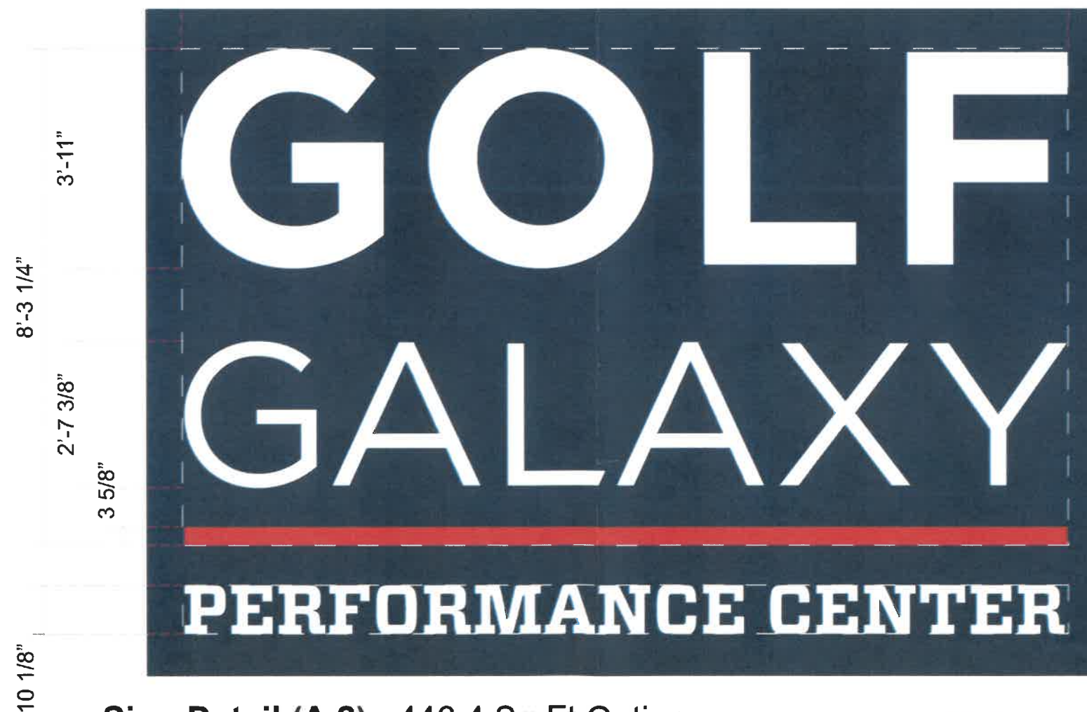
Sign Detail (A.2) - 446.4 Sq Ft Option Scale: 3/8" = 1'-0"
