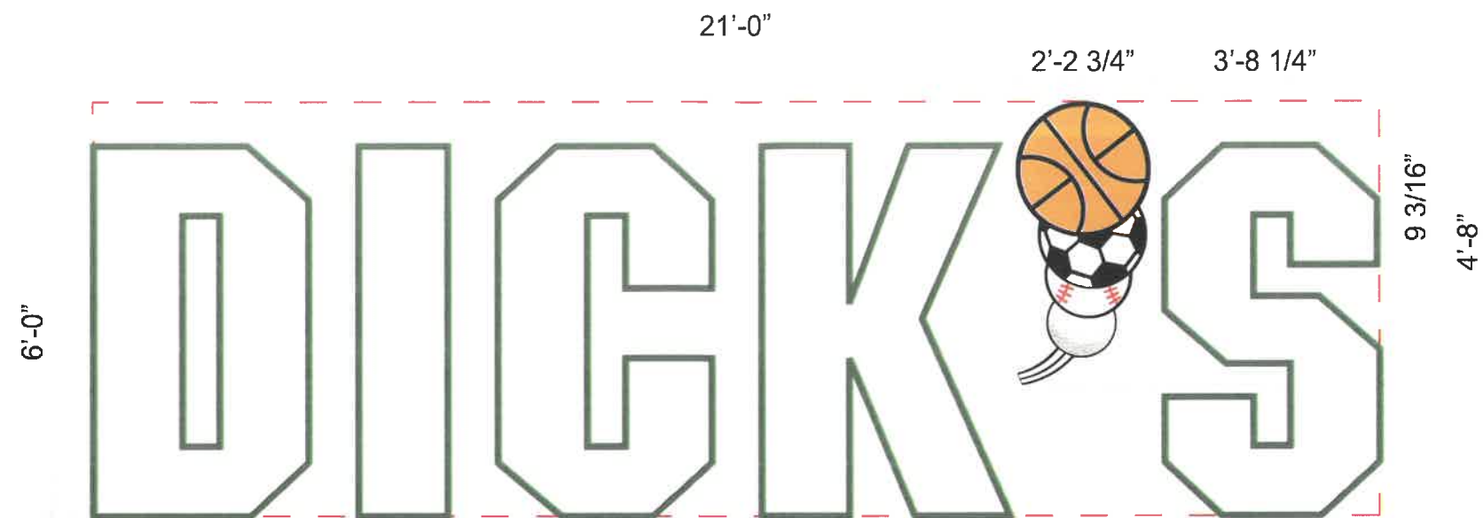
Sign Detail (A.1) - 200 Sq Ft Option Scale: 3/8" = 1'-0"
