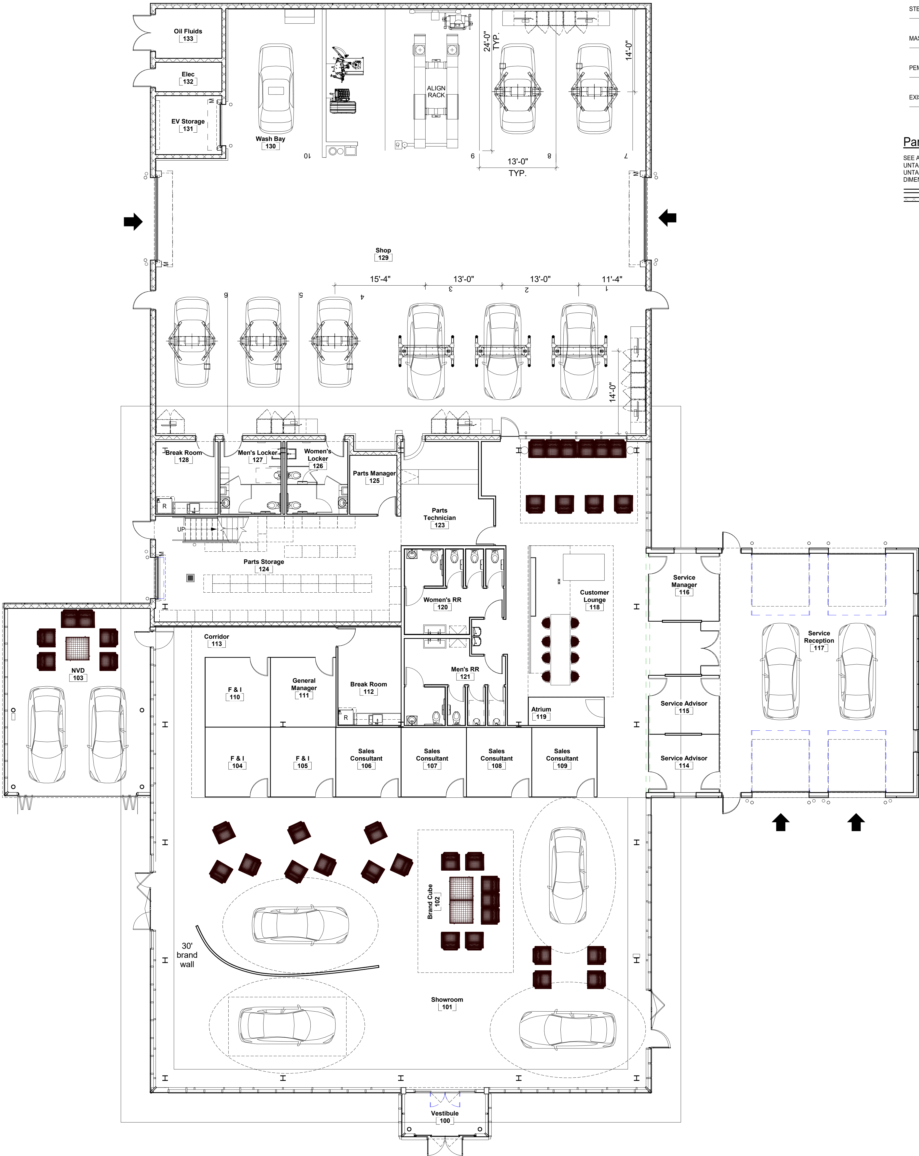
0 4 8 16 32 PROJECT NORTH 1 A201 1/8" = 1'-0" First Floor Plan - Overall
