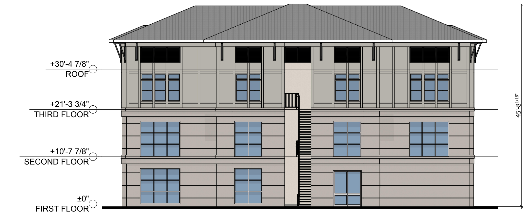
1 SOUTH ELEVATION A5-5.1 SCALE: 3/32" = 1'-0"
